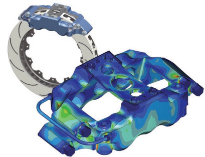
Pro/ENGINEER Mechanica enables validation of designs, such as this model of a brake, and reduces the number of physical prototypes needed.
